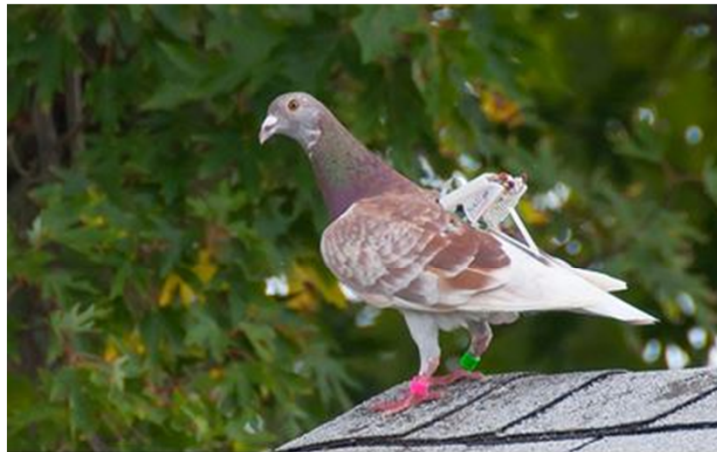
A backpack with piezoelectric material generates energy from the motion of a bird's wings in flight. (Photo courtesy of Michael Shafer)
