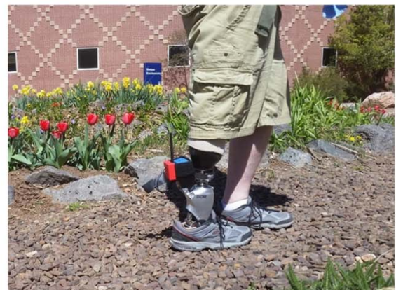
Prototype foot/ankle prosthetic uses CBI actuator technology.
